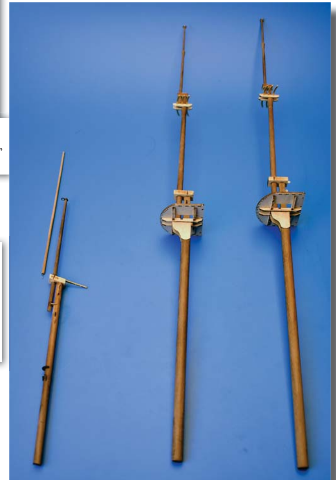
Right - Bowsprit, fore and mast masts built up. Note the pin in the end of the flying jibboom (the unattached slim long tapered dowel next to the bowsprit). This pin will be fixed into the front face of the bowsprit cap to secure the part.
