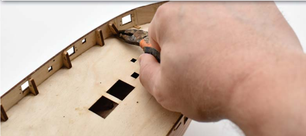
18 - Remove all bulkhead tabs above deck level by carefully bending and twisting with a pair of pliers or similar. Once removed, sand any remaining stubs flush with the deck.
